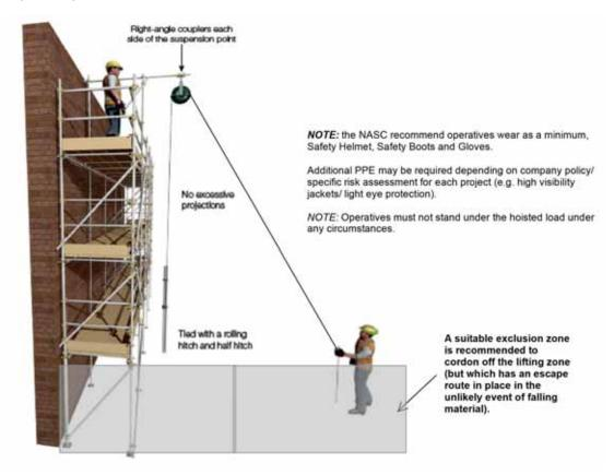
*NOTE:* there are proprietary Gin Wheels on the market with specialist differences (such as an integral brake system, which prevents the rope travelling when the brake is applied).
