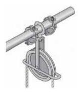
NOTE: load bearing double couplers MUST be fixed either side of the Gin Wheel.
