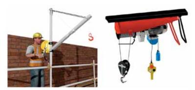
Wherever a jib crane is used to lift loads greater than 50 kg, consideration should be given to the need for the scaffold to be strengthened at the location of the crane and additional or stronger ties to the building provided, following guidance from the manufacturer or from a scaffolding designer.
