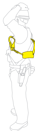
(iii). A hybrid self-retracting lanyard with minimum trailing lanyard when stowed.
