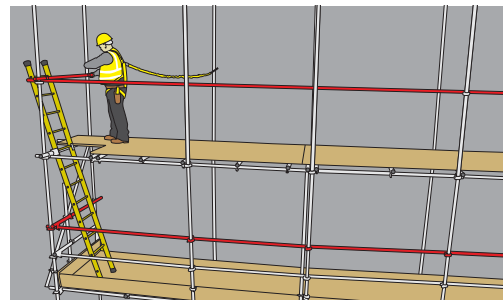
(iii) Progressively install guardrails (including stop-ends etc.) remaining continually attached to create the scaffolders' safe zone .
