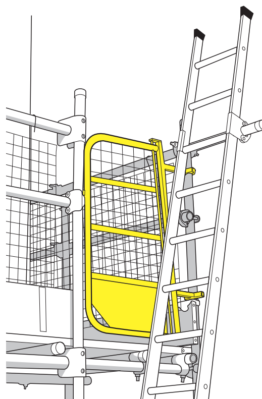
Figure 60: External ladder access using a safety gate as an example of good practice.
