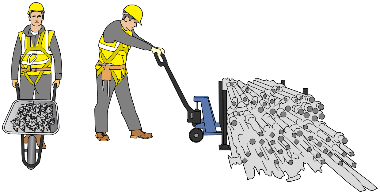
Fig. 9 Pallet trucks and wheelbarrows are examples of manual handling aids used in scaffolding operations.
