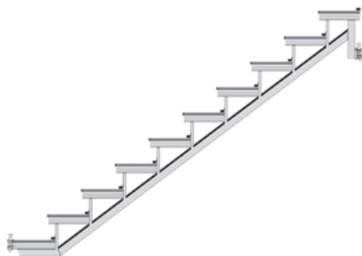
U-stairway stringer 200, 10 steps, 2.00 m storey height, Ref. No. 2638.010, 2.00 x 2.57 m
