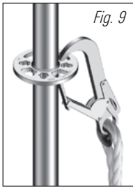
Fig. 9: Attachment in large and small hole of rosette possible (Only permissible in Allround Scaffolding in steel – not in Allround Scaffolding in aluminium) Fig. 10: Attachment points to Allround O- / U-ledgers; maximum bay length 3.07 m
