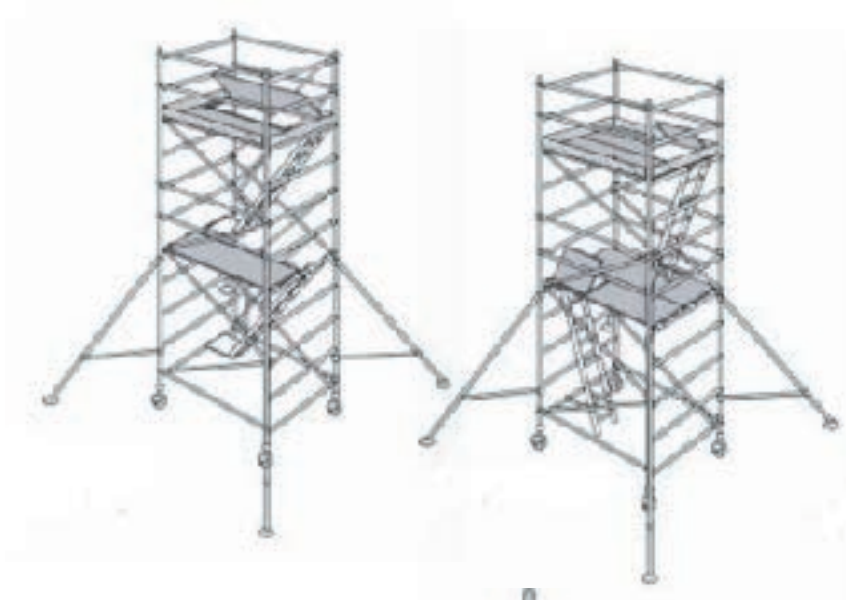
Figure 21: Example of Mobile Towers with Ladder Access and with Stairway/Stair-ladder Access (From PASMA)
