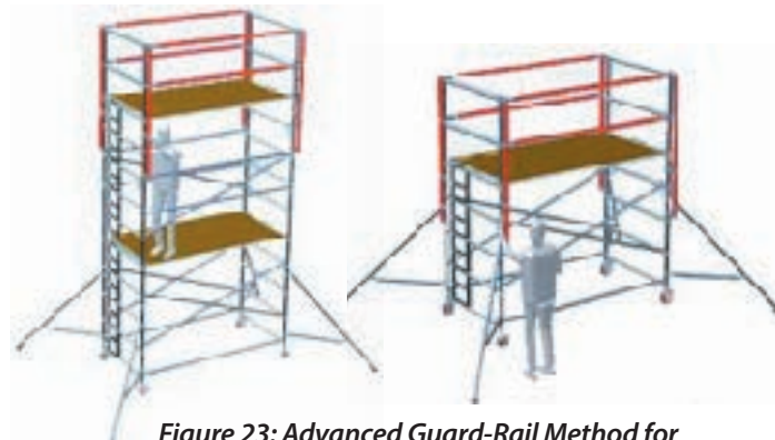
Figure 23: Advanced Guard-Rail Method for Erection of Mobile Towers (From PASMA)
